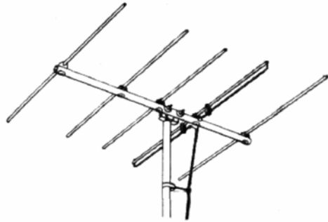
Figure 28.2: A Yagi-Uda antenna was invented by heuristics in 1926. The principal element of the antenna is the folded dipole. When a wire dipole antenna is less than half a wavelength, it acts as a waveguide, or a director. When the wire antenna is slightly more than half a wavelength, it acts as a reflector [136]. Therefore, the antenna radiates predominantly in one direction (courtesy of Wikipedia [137]).
